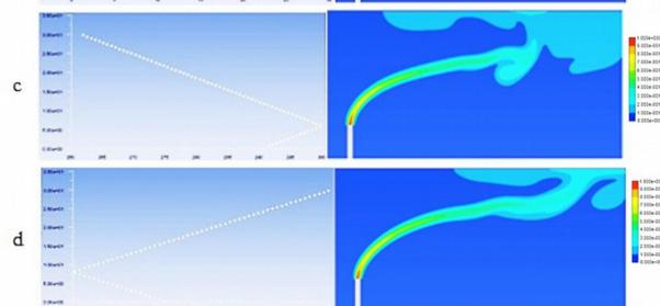
Figure 8 – Methane ( $CH_4$ ) concentration distribution for various initial temperature profiles in case when pollutant-emission rate is 4 m/s
