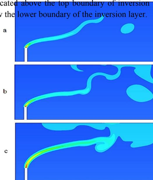
**Figure 4** – Methane ( $CH_4$ ) concentration distribution in case when the source mouth is located above the upper boundary of inversion layer
