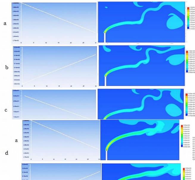
**Figure 7** – Methane ( $CH_4$ ) concentration distribution for various initial temperature profiles in case when pollutant-emission rate is 4 m/s
