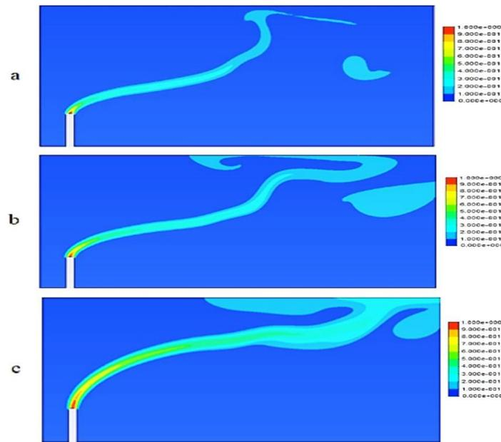
**Figure 5** – Methane ( $CH_4$ ) concentration distribution in case when the source mouth is located below the lower boundary of inversion layer
