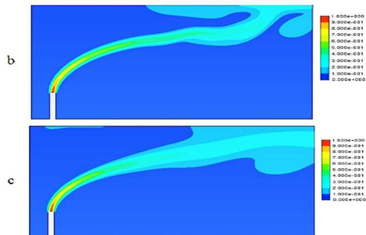
**Figure 9** – Temporal distribution of methane ( $CH_4$ ) concentration in case when the lower boundary of inversion is located above mouth of source
