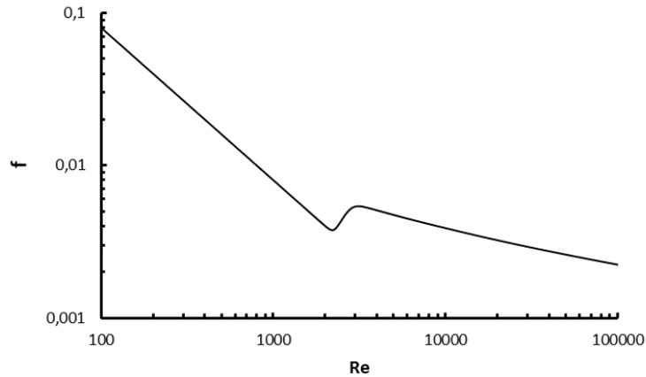
FIGURE 4: Friction curve given by Churchill's model [8].
