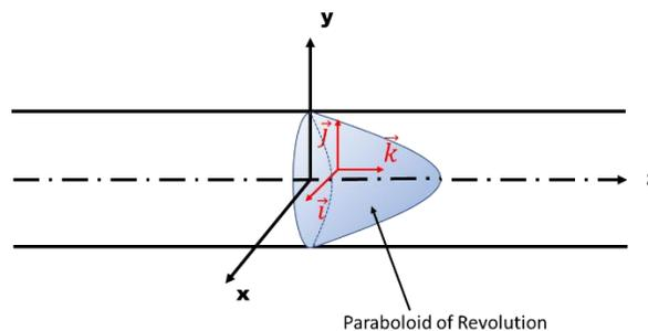
FIGURE 1: Laminar flow velocity field giving a paraboloid of revolution.
