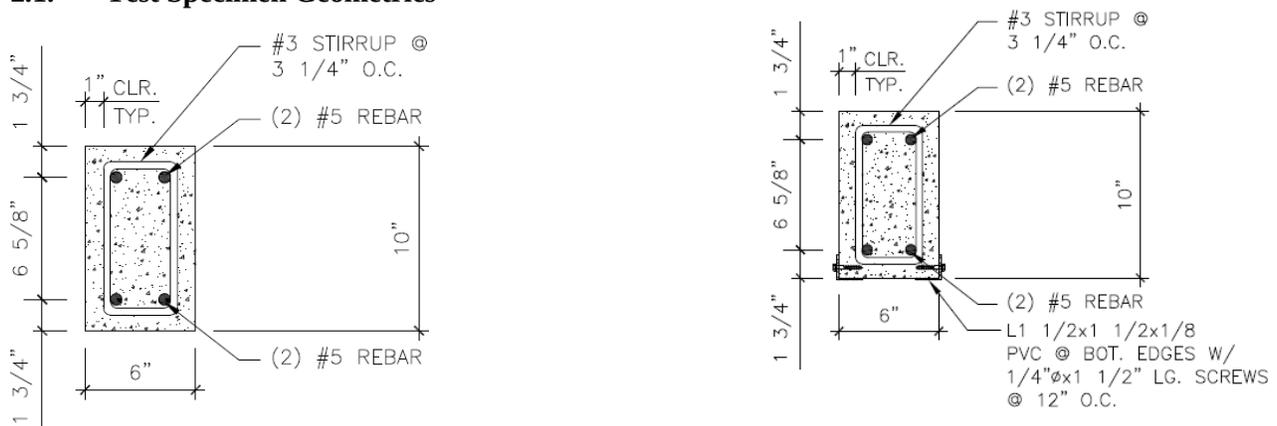
Figure 1. Cross section of (a) Beam 1 and (b) Beam 1R and Beam 2. (1 in. = 25.4 mm)
