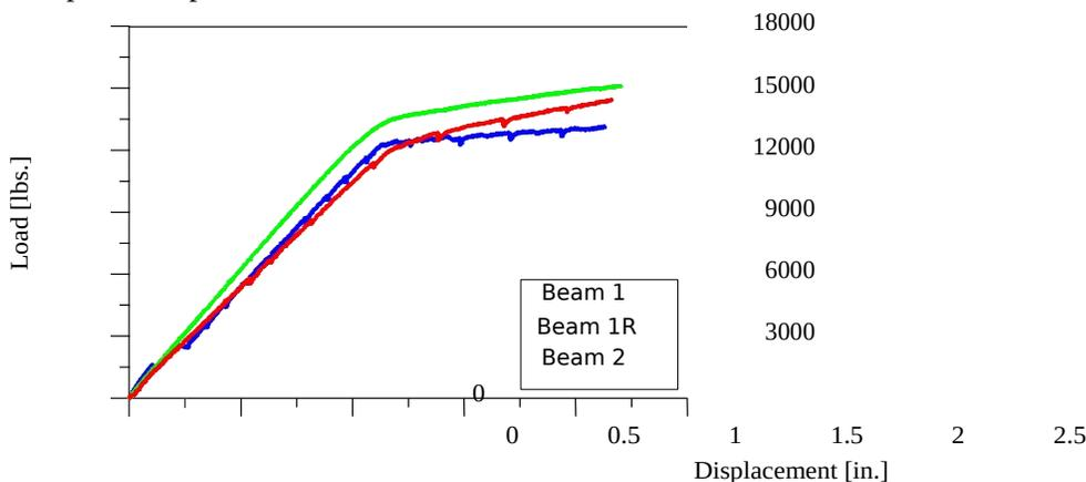
**Figure 8.** Experimental load-displacement results for Beam 1, Beam 1R, and Beam 2. (1 in. = 25.4 mm, 1 lb. = 4.45 N)
