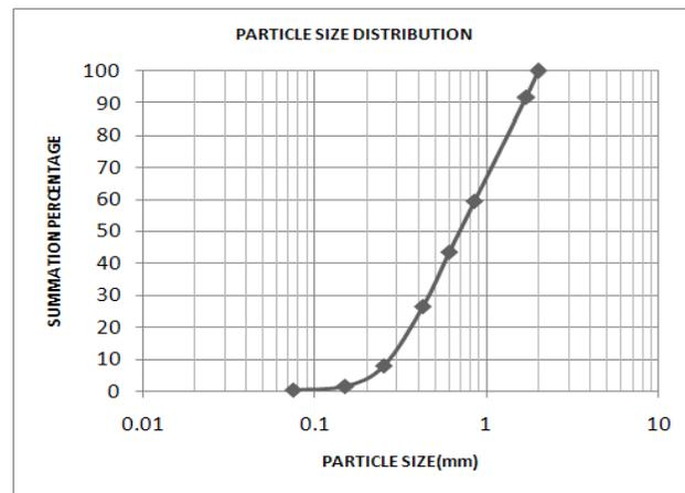
**Figure 3.** The grading curve of used sand
