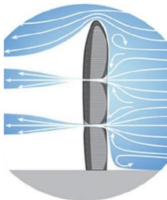
**Figure 6.** Pearl River Tower showing the functioning of wind turbines
