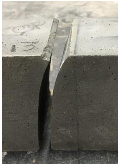
**Fig. 9: Typical crack patten for the unreinforced MOR specimens**
