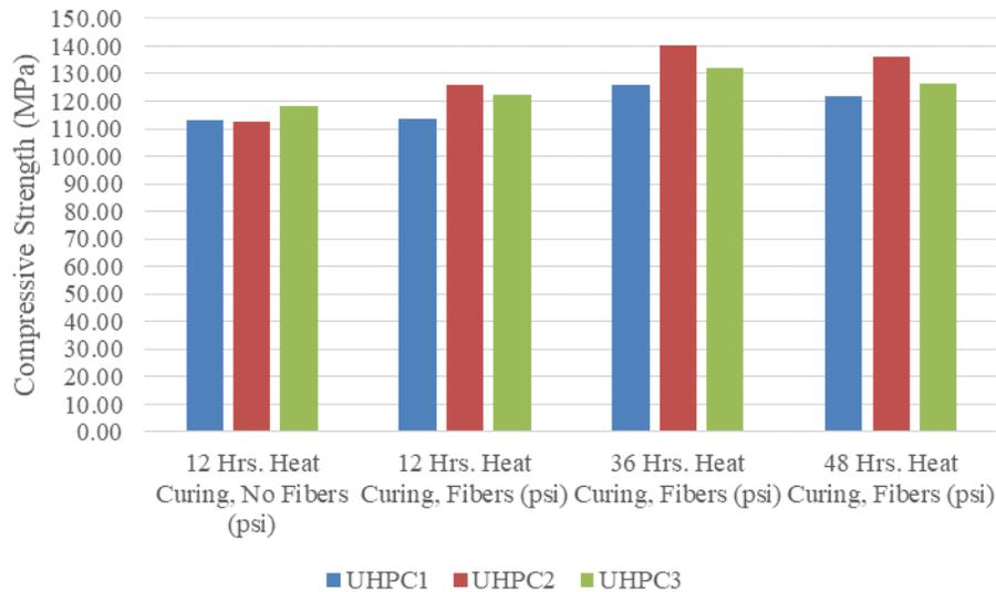
**Fig. 7: Compressive strength test results with fibers**
