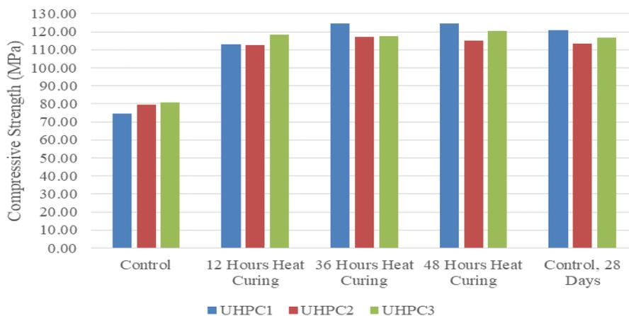
**Fig. 6: Compressive strength test results without fibers**
