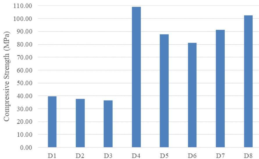
**Fig. 4: Series D compressive strengths**
