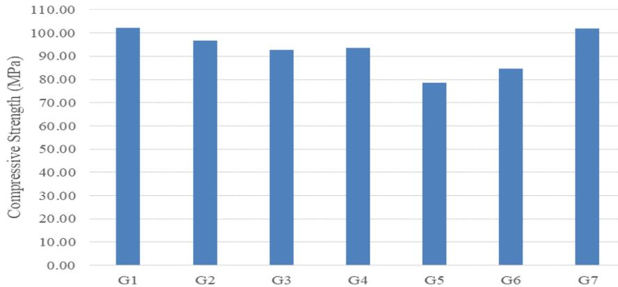
**Fig. 5: Series G compressive strengths**
