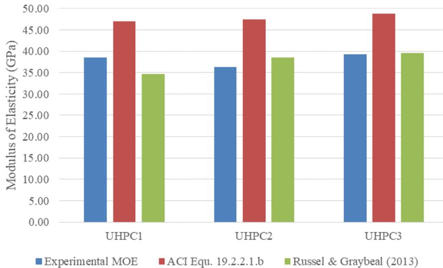
**Fig. 10: MOE test results plot**
