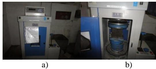
Figure 3.1: a) Digital compression machine during cube testing for compressive strength and b) a sample during compression testing
