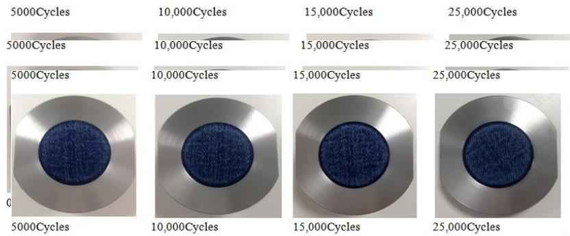
around the last example than in the first reused test, in spite of the fact that it isn't as wide as the different as in the main example. The exchange to the abradant texture is significantly more than in the primary example taken from the reused denim. The manner by which the color has blurred is inconsistent yet like every one of the examples taken there is no fluffing or harm to the texture.
