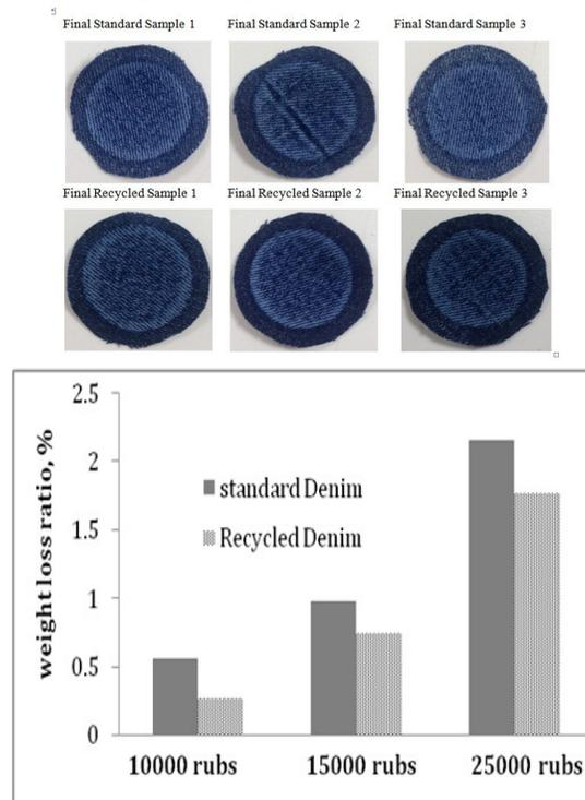
**Figure 1** Weight loss comparison between standard and recycled Denim.
