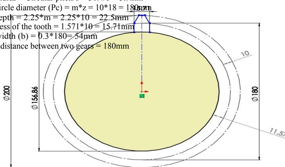
**Fig.01** Gear calculation
